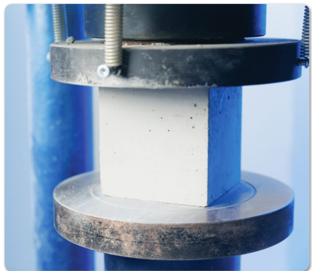
Compressive strength testing of concrete specimens
